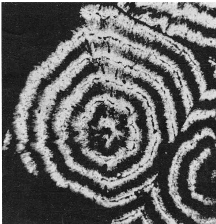
Fig. 9. Spherulite structure produced in polyoxymethylene resin on repeated melting. Scale: 1\frac{1}{4} in. = 1 mm.
